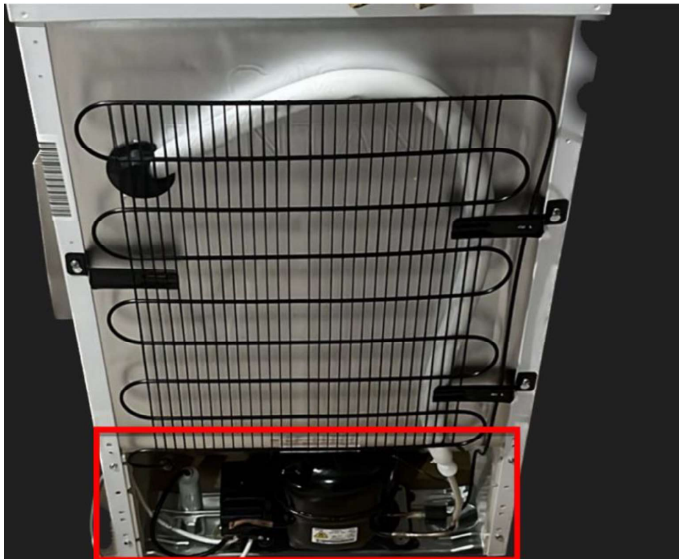
Figure 3.9 Montaged view of the compressor
