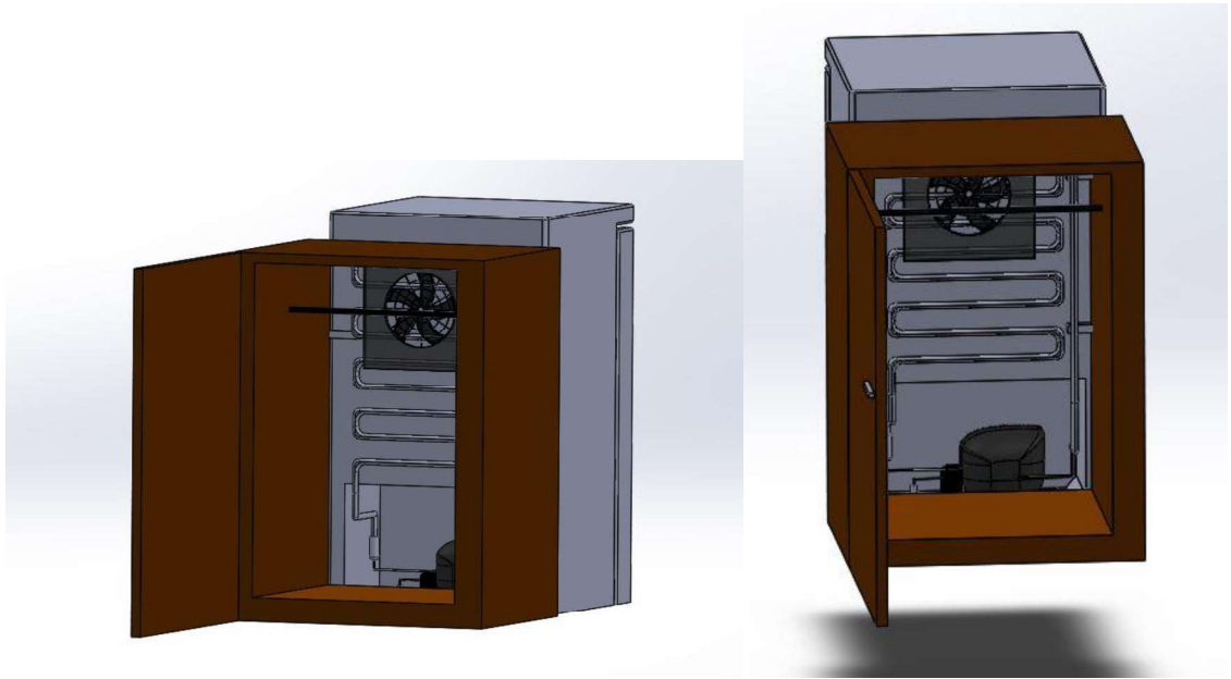
Figure 7 The view from different aspects of fan from above designed system Figure 7 is about the experimental setup for Test Step 4.a and Step 6. The fan is assembled above position. The setup helps to determine the most efficient design.
