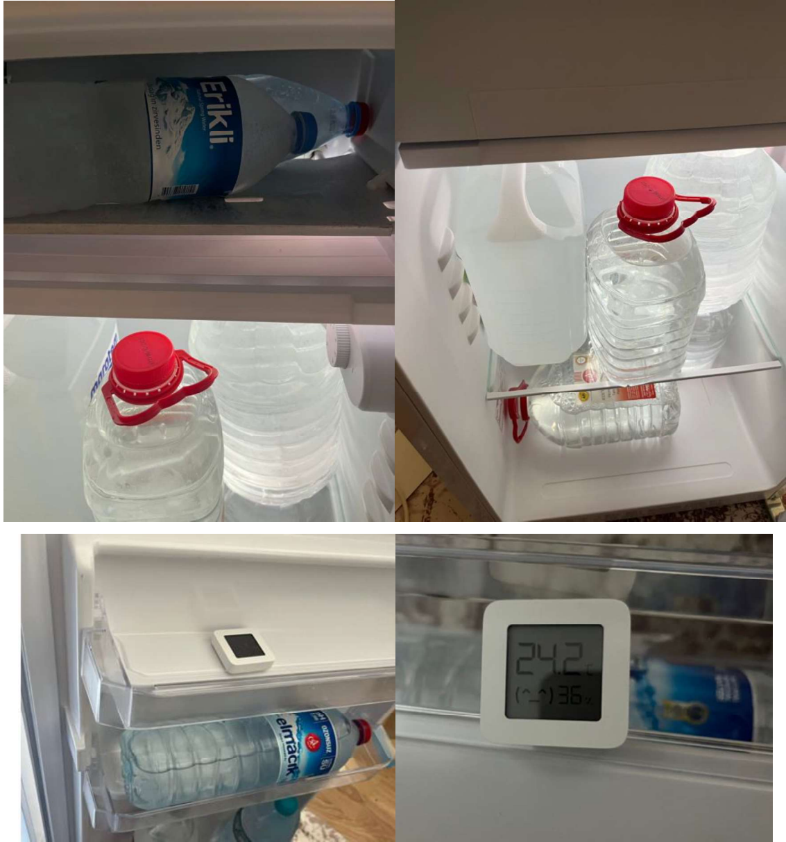
Figure 2.. 20,5 L + 3 L water and temperature sensor placing
