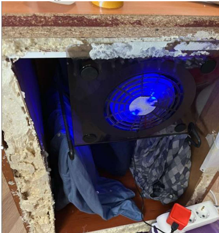
Figure 3. Insulated clothes dryer chamber with fan from above
