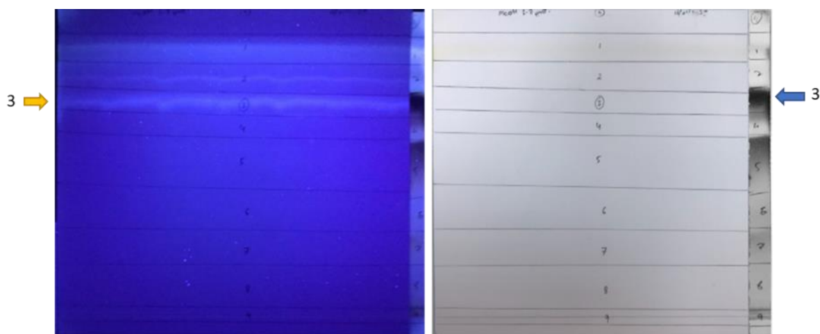
Figure 4.24. TLC analysis of chloroform-insoluble B fraction (images captured under UV-366 nm and normal light after acid charring).
