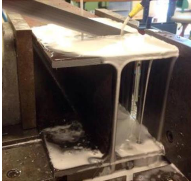
Figure 3.6. The representative view of the initial cutting process of the beam [93].
