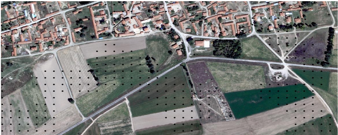
Figure 4.28. The orthophoto has been overlaid with EUDEM ground points.
