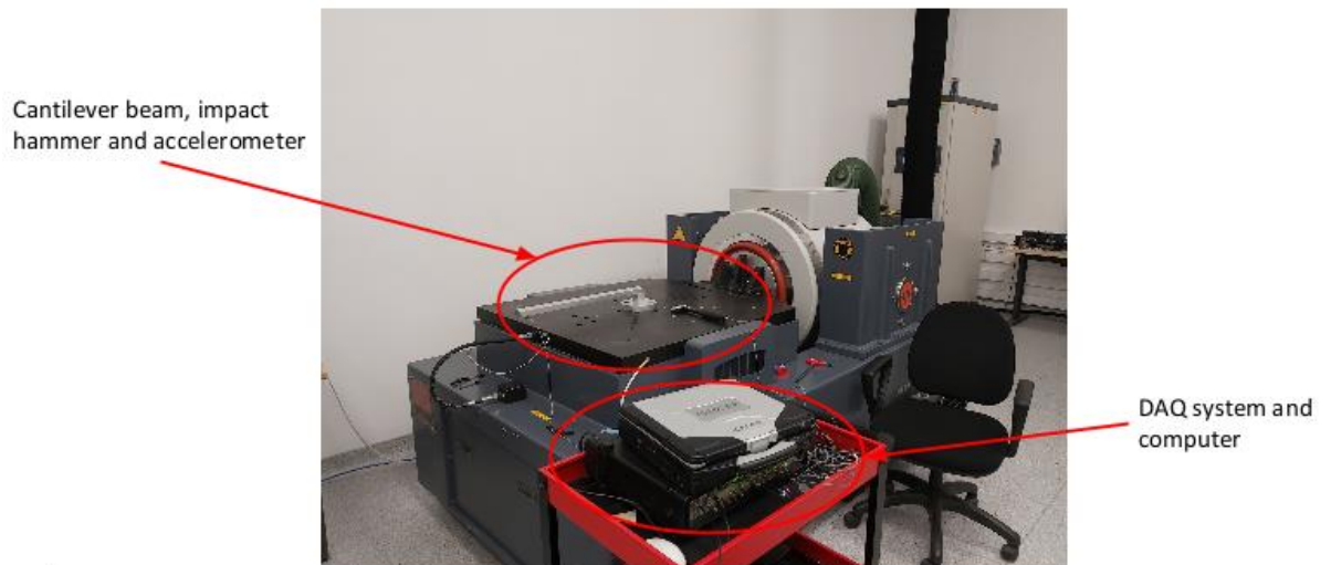
Figure 5.1 Cantilever beam characterization test setup
