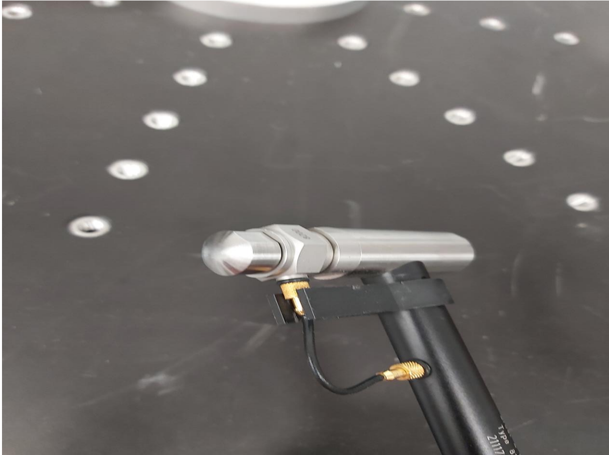
Figure 5.2 Impact hammer with hard tip
