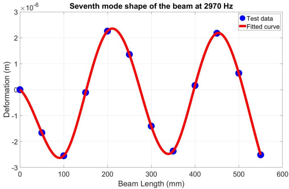
Figure 5.15 Test result for 7th mode shape of the cantilever beam
