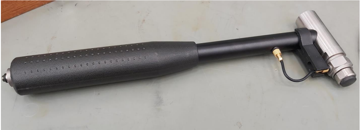
Figure 5.22 Impact hammer with soft tip
