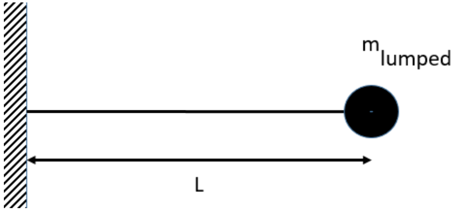
Figure 2.13 Schematic illustration of a cantilever beam that is modeled with lumped mass.
