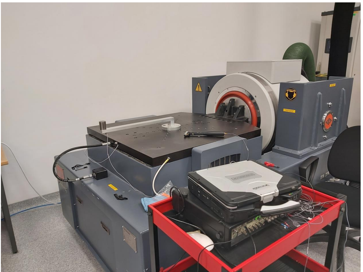
Figure 5.23 Cantilever beam characterization while the TMD is off test setup
