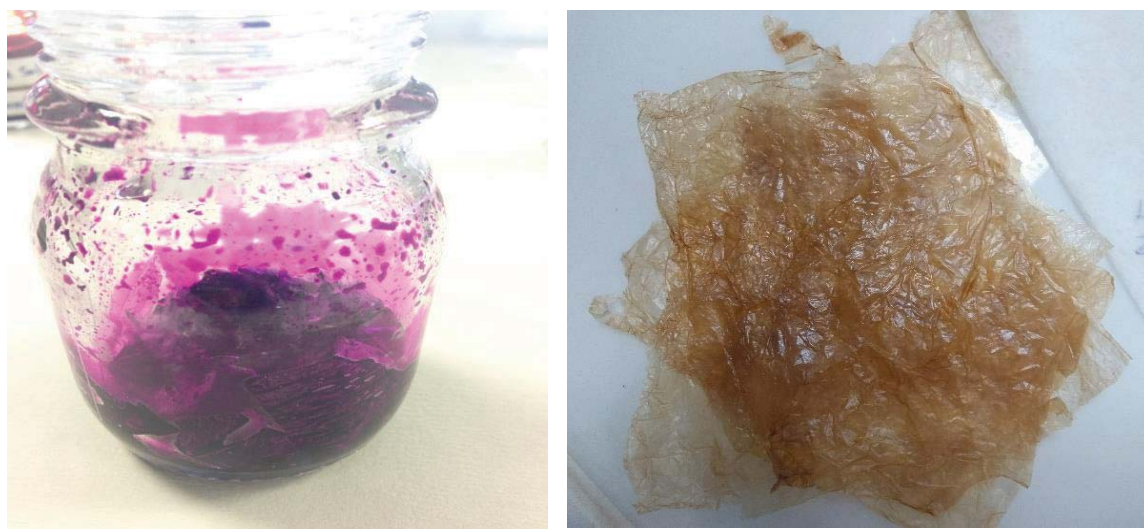
Figure 2.2. PE samples with \text{KMnO}_4 inside the bottle before (left) and after (right) microwave exposure.
