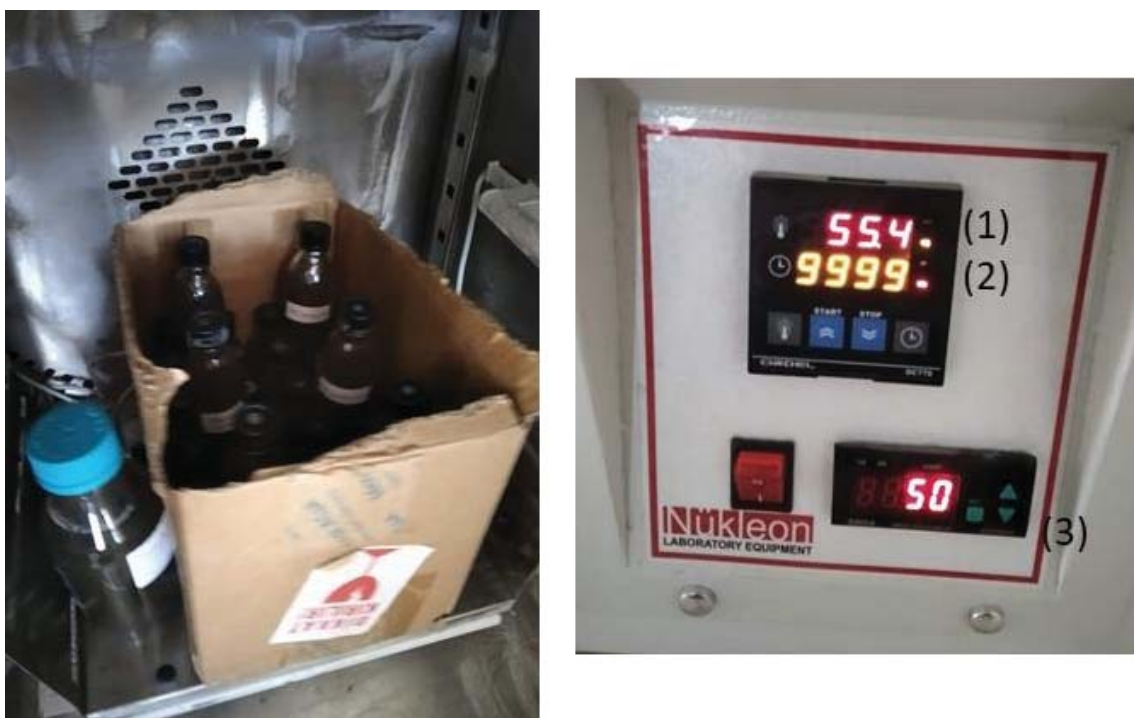
Figure 2.5. Bottles placed in the incubator (left). Incubator's controllers and display of temperature (1), time (2) and agitation (3) (right).
