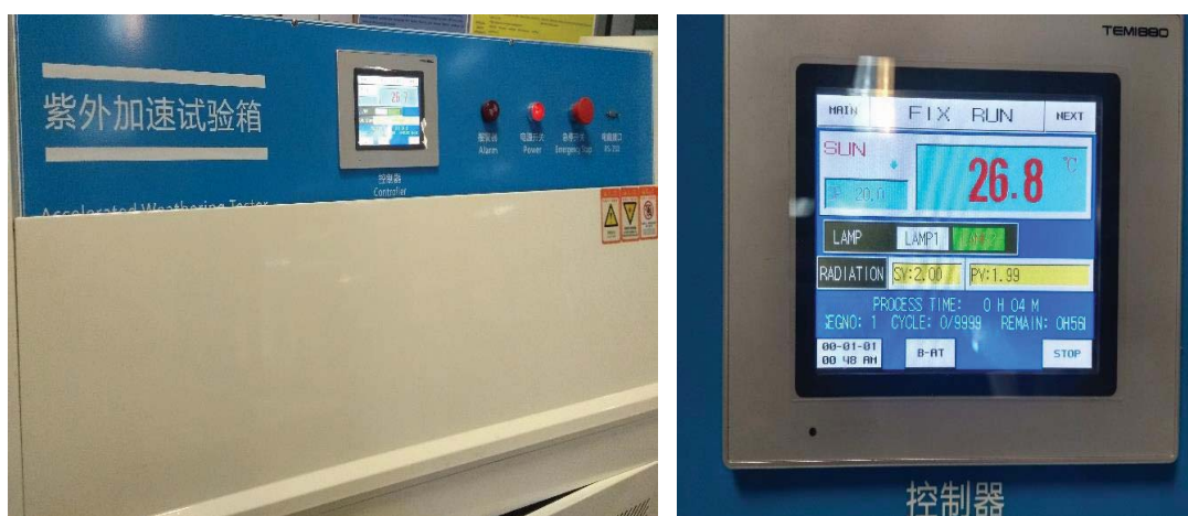
Figure 2.1. Accelerated Weathering Tester and programmable controller.
