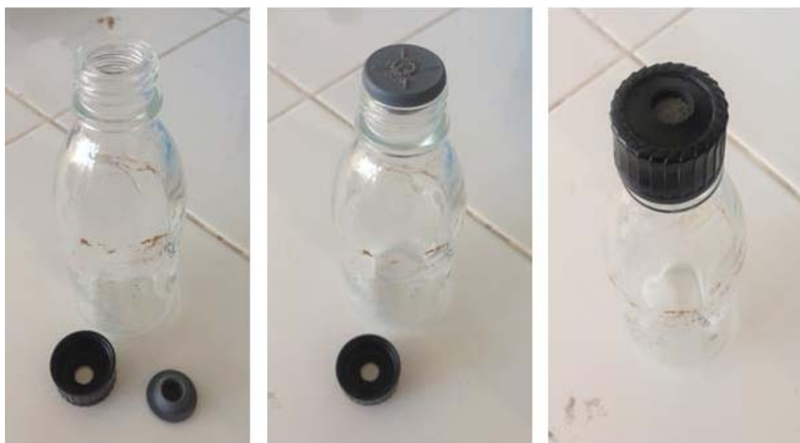
Figure 2.4. Bottles used for anaerobic degradation.
