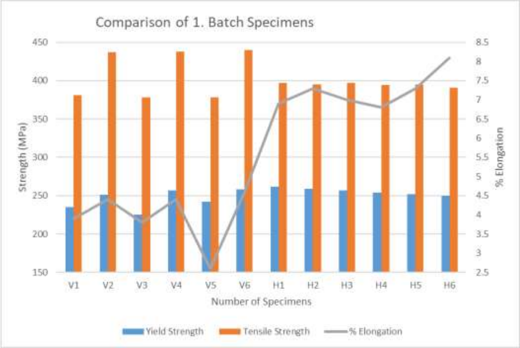
Figure 5.5 Strength vs Specimen Numbers for AlSi10Mg Material
