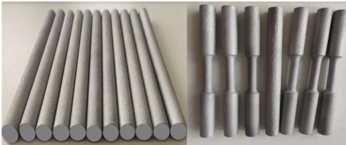
Figure 5.2 Cylindrical Shaped and Dog Bone Shaped Test Samples
