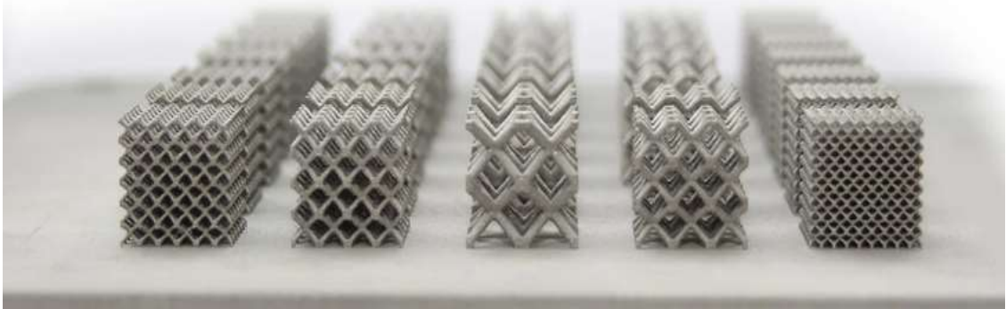
Figure 2.9 3D Printed Lattice Structures Demonstration [6]
