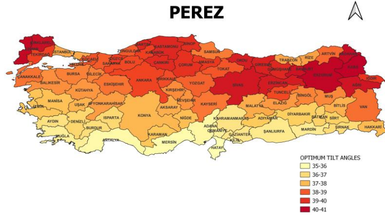
Figure 40 The Map Modelling of Annual Optimum Tilt Angles of Turkey by Perez Model
