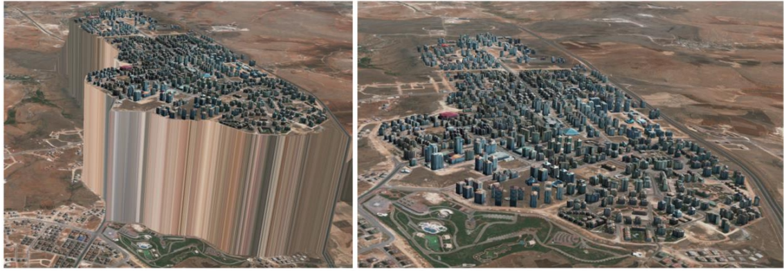
Figure 6.1 A view of Cesium World Terrain unmerged (left) and merged (right) high-resolution DTM
