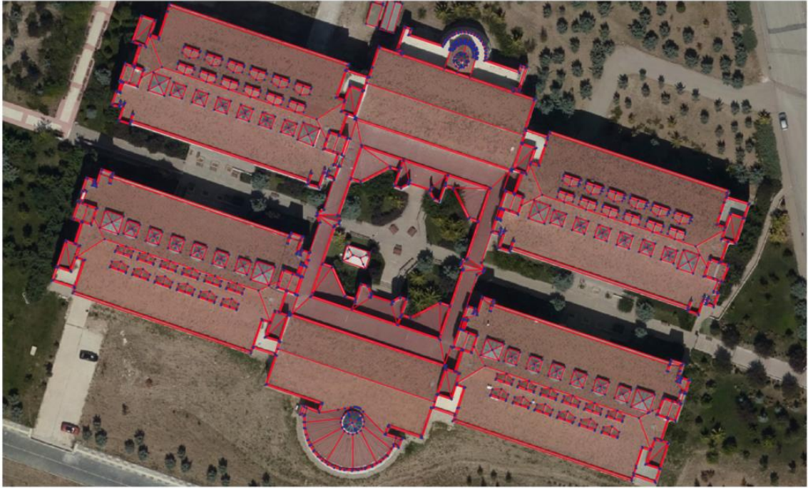
Figure 5.2 A close view of complex LoD2.2 building roof structure
