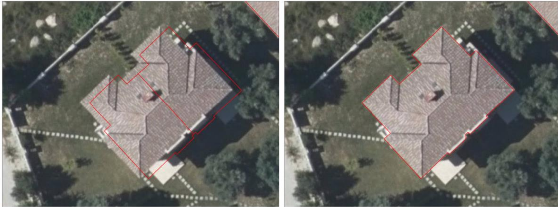
Figure 4.2 An example of a roof vector before (left) and after (right) correction
