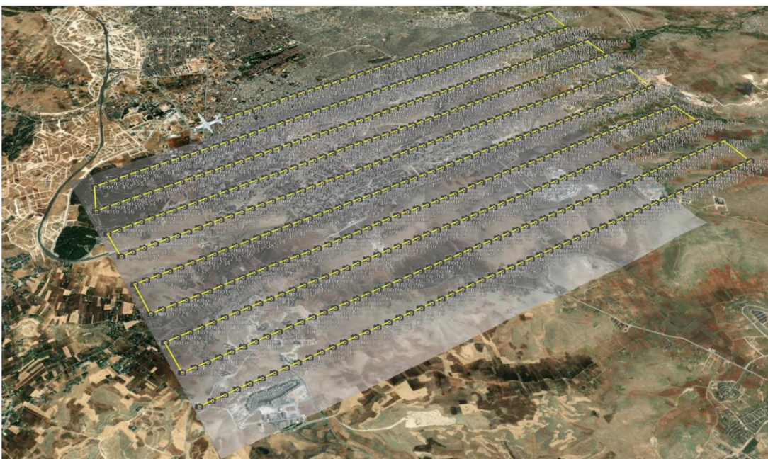
Figure 6.11 Photogrammetric image acquisition of 736 images in Gaziantep, Turkey with an 80% forward and 60% lateral overlap [58].
