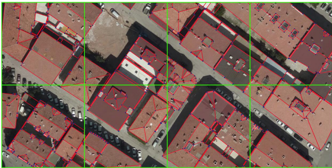
Figure 5.10 Merged roof structures of 8 image tiles.
