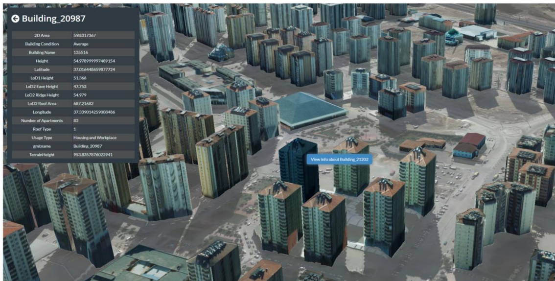
Figure 6.5 A view of attributes for selected LoD2 building in the web interface
