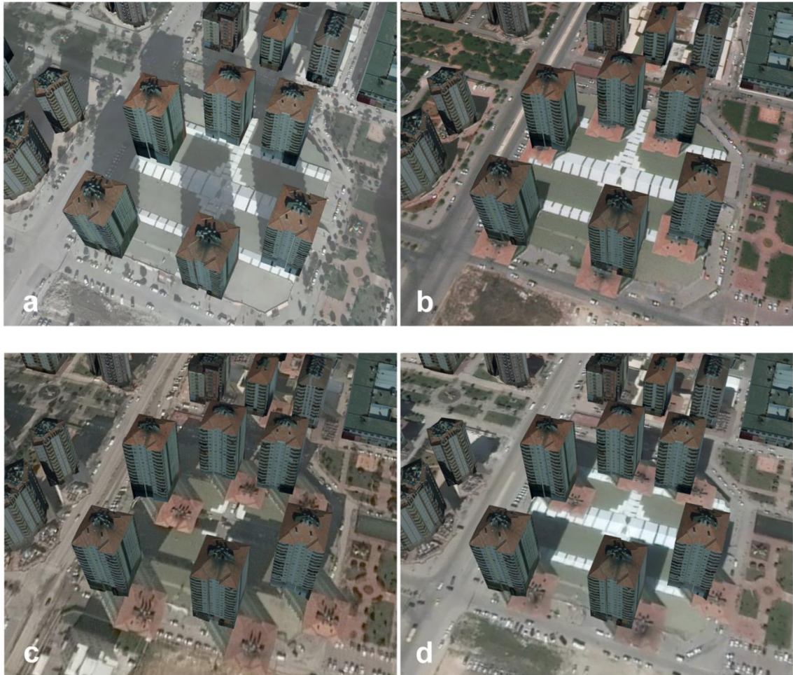
Figure 6.4 A comparison between true orthophoto (a), Bing Maps (b), Mapbox Satellite (c), and ESRI World Imagery (d) as basemap layers
