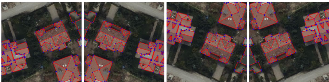
Figure 5.5 Augmented files with ground truth a. original file, b. horizontal flip, c. vertical flip, d. mirroring
