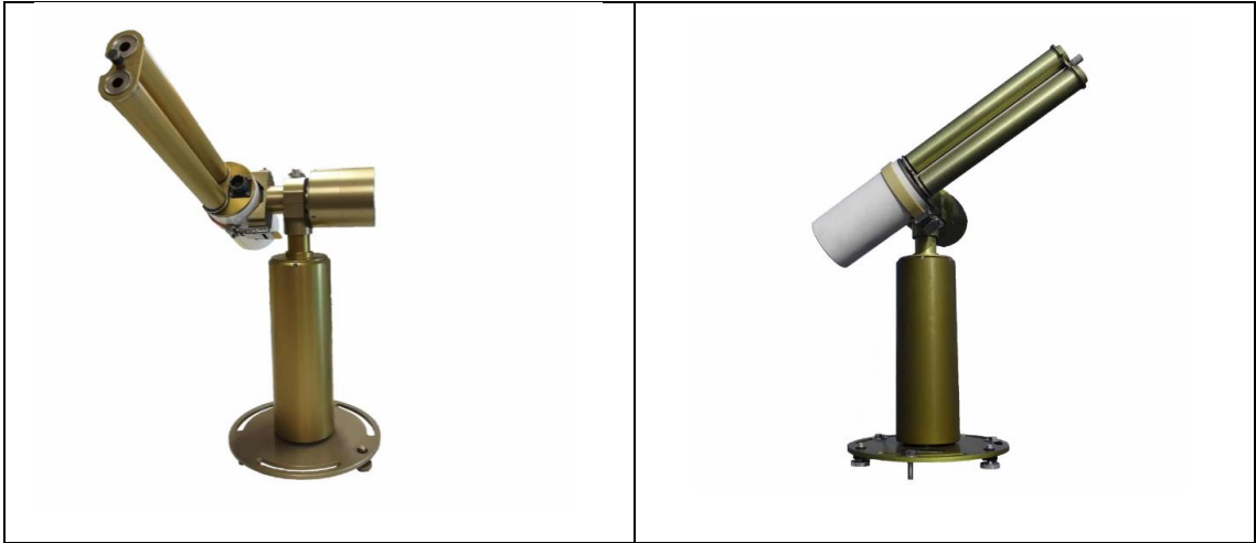
Figure 2.3. CE318 photometers( CE318-T - Sun Sky Lunar Multispectral Photometer | Cimel Electronique, n.d. )
