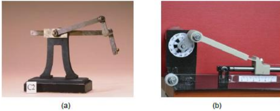
Figure 3: Rigid (a) and compliant arm-slider mechanism (b) [3].
