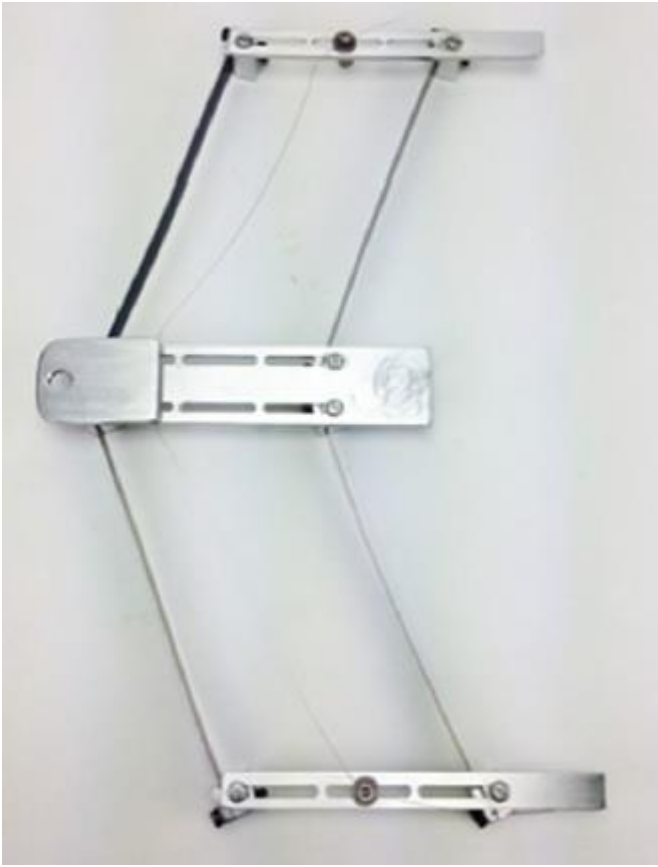
Figure 8: Compliant constant-force linear-motion mechanism [13].
