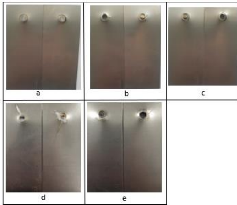
Figure 23. Fracture type of triple pulse welding a)7.2 kA b)8.4 kA c)9 kA d)10 kA e)11kA
