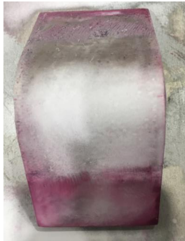
Figure 5.9 6mm Aluminium with R12mm – Liquid Penetrant Test
