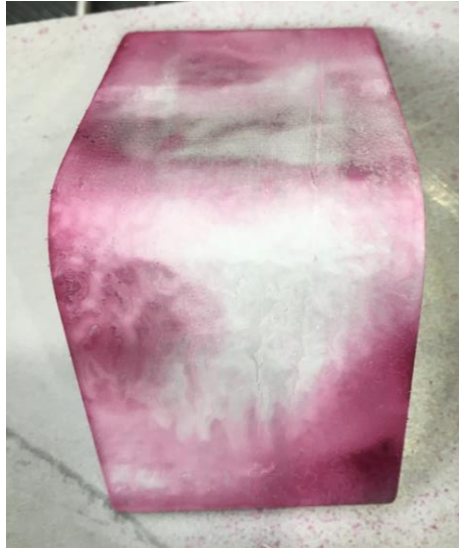
Figure 5.6 4mm Aluminium with R8mm – Liquid Penetrant Test
