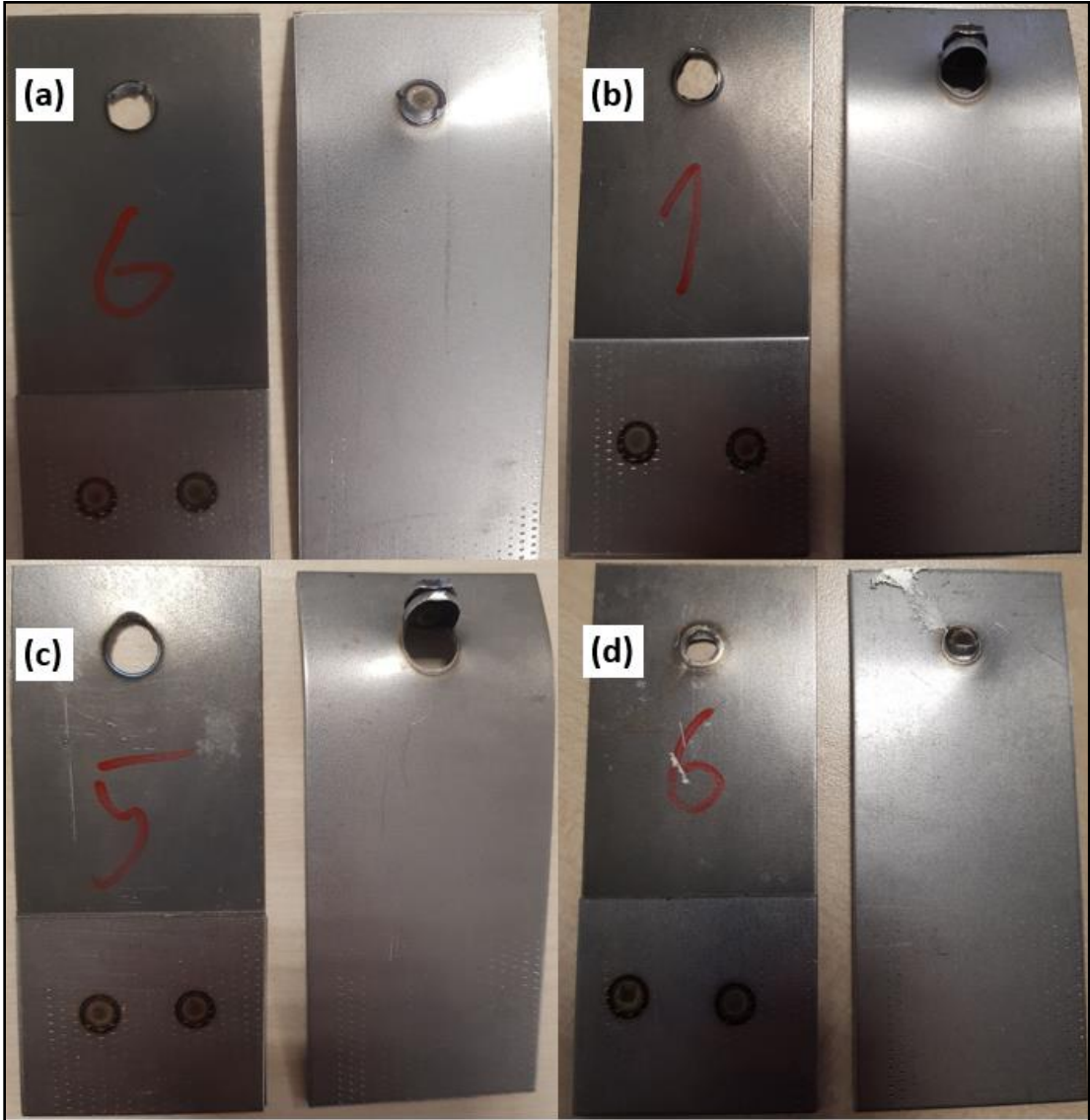
Figure 4-2: Failure modes of resistance spot welding samples (a) interfacial failure (single pulse 8.8 kA) (b) pullout failure (8.8 – 7.2 kA) (c) pullout failure followed by base metal tearing (8.8 – 8.4 kA) (d) pullout with expulsion (8.8 – 9.2 kA)
