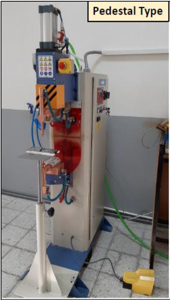
Figure 3-3: Pedestal type AC resistance spot welding machine used in study
