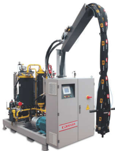
Figure 22 Low- and High-Pressure Dosing Machine Developed by Canon Afros Company [23]
