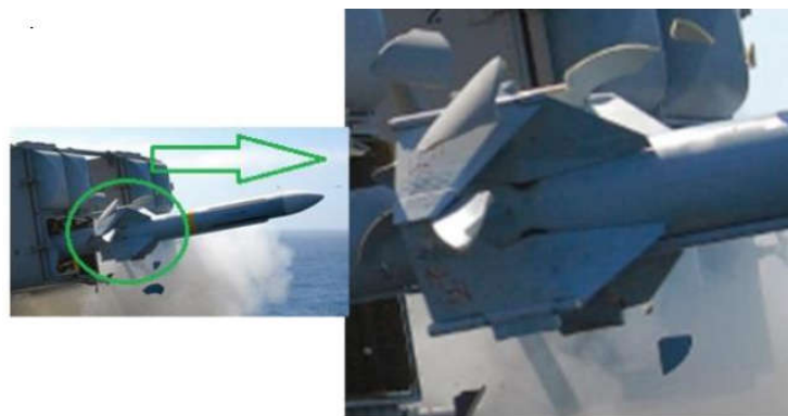
Figure 6 Broken Foam Canister Cover Parts Belongs to Sea Sparrow Weapon System
