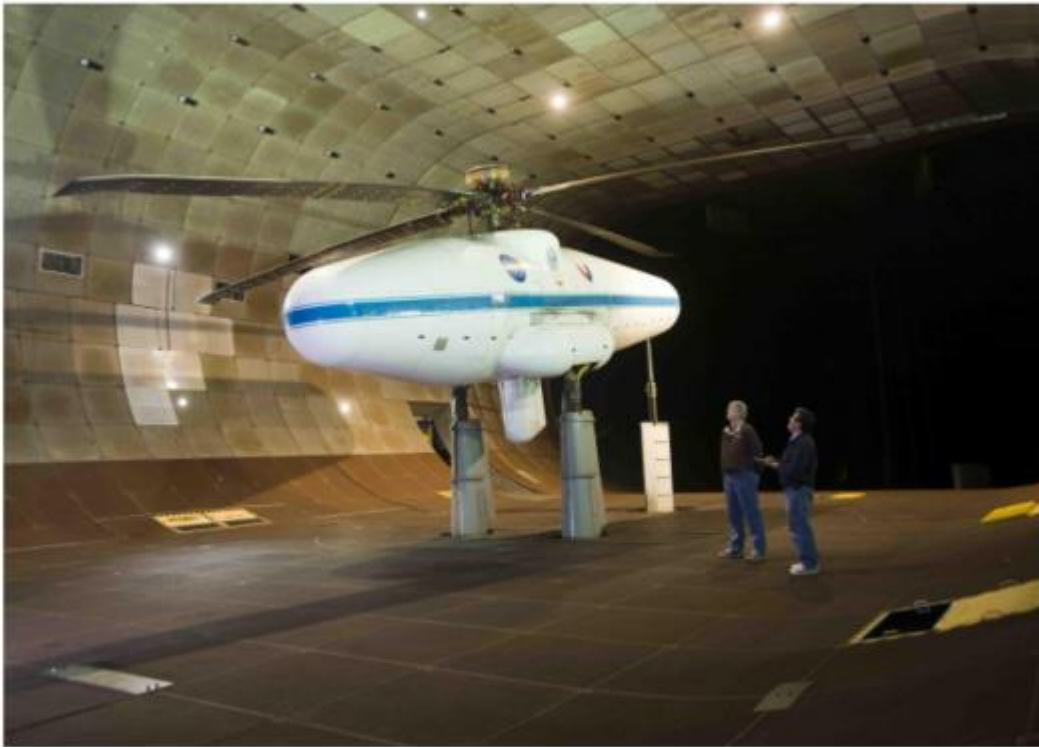
Figure 9: UH-60 Blades in NASA Ames 40-by 80-foot Wind Tunnel [11]
