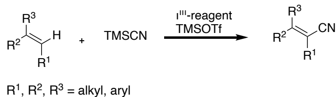
Figure 2.18. Synthesis of acrylonitrile by direct metal-free cyanation of alkene
