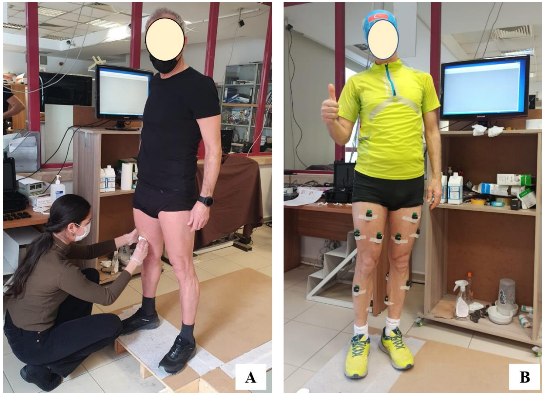
Figure 3.3. (A) Representative scene of skin preparation for sEMG measurement, (B) Representative sEMG electrode placements for ventral muscles.
