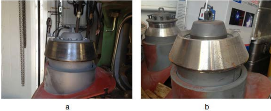
Figure 3-10. Shear (a) and shear-free (b) rollers for LM 4,5.4
