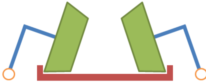
Figure 2-26. Loesche type roller table layout [16]
