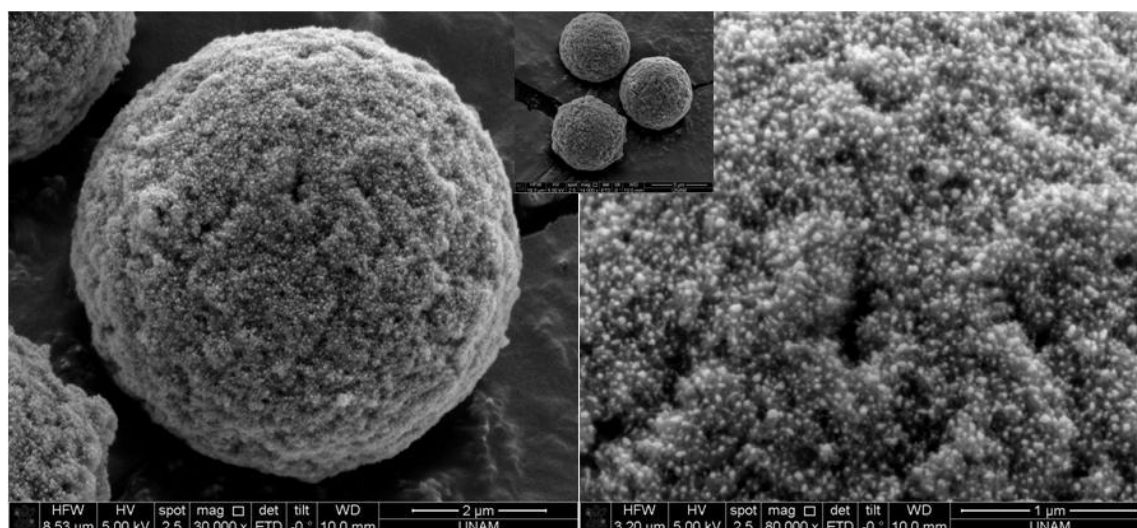
Figure 4.19. SEM photograph of monodisperse-porous Turkevich AuNP decorated magnetic titania microbeads with an Au loading of 5.0 % (%w/w).
