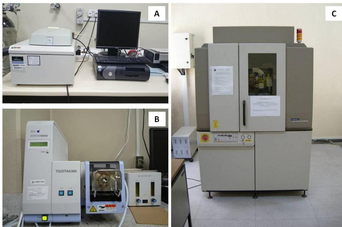
Figure 3.11. Devices used for the characterization of poly(HPMA-Cl-co-EDMA) microbeads (A) DSC, Diamond DSC, Perkin Elmer, (B) TGA, TG/DTA 6300 SII EXSTAR 6000, Perkin Elmer, (C) XRD, Rigaku, D/Max-2200.
