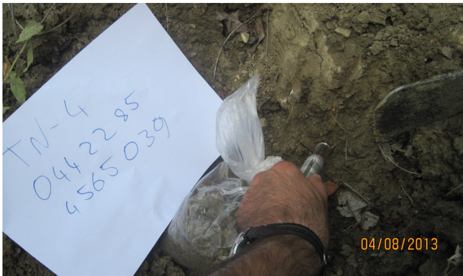
Figure 4.1: Determination of soil strength with pocket penetrometer and soil sampling in plastic bag
