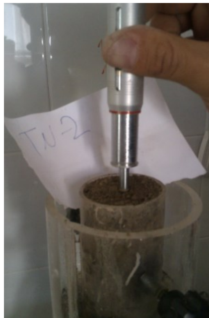
Figure 4.6: Testing apparatus and determination of compactness
