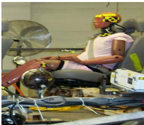
Figure 2. A Test setup for BIORID II DUMMY [27]
