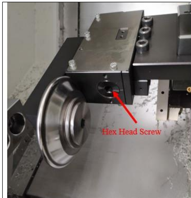
Figure 19 Deep Rolling Tool and Hex Head Screw to Load Spring within
