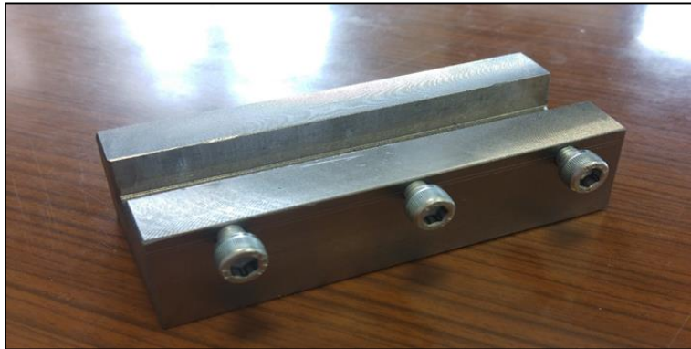
Figure 20 Fixture Designed to Manufacture Flat Surface Specimen
