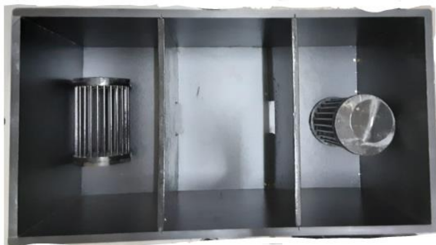
Figure 3.7. Three-chamber social memory protocol and apparatus (the left cylinder was laid for the demonstrative purpose only).
