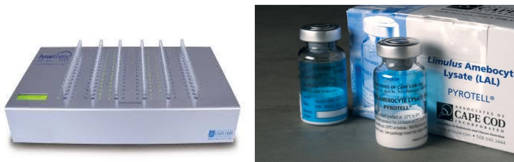
Figure 2. 3. Pyros Kinetix® Flex tube reader and Limulus Amebocyte Lysate (Pyrotell®-T)
