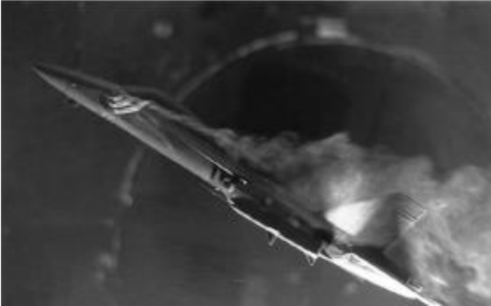
Figure 1.5. Tail buffeting of F-18 [7]
