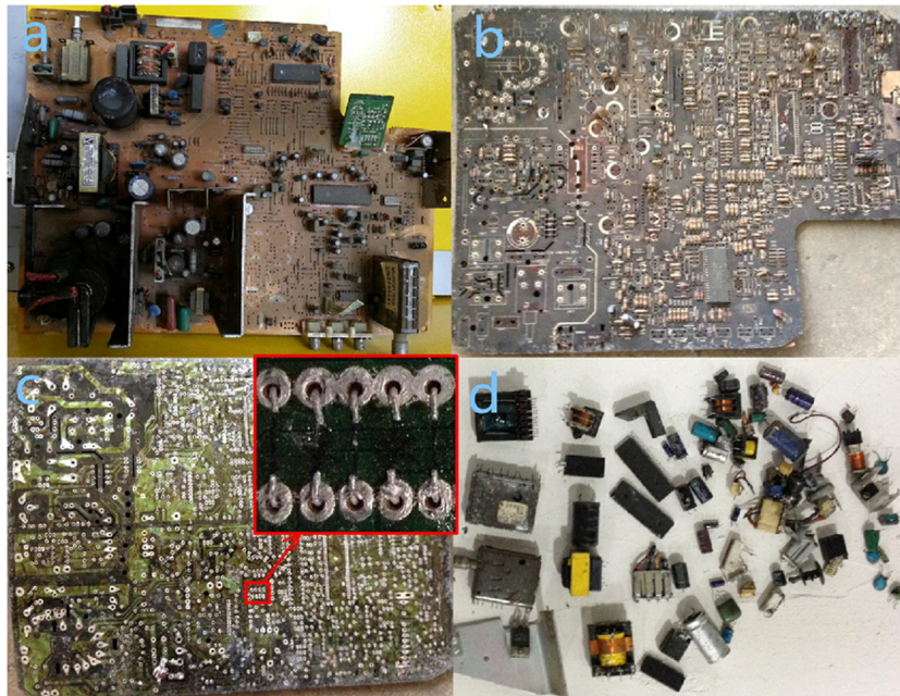
Figure 2.5. Photos of the TV-WPCB: (a) TV-WPCB (b) front side of the TV-WPCB after dismantling, (c) back of the TV-WPCB after dismantling, and (d) dismantled electronic components [63]
