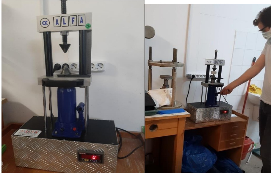
Figure 37. A view of the test setup of the point load test.
