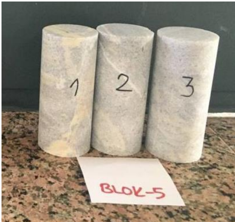
Figure 30. The view of the TCS test core samples having marble lithology
