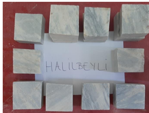
Figure 38. A view of the point load box samples prepared from the marble blocks
