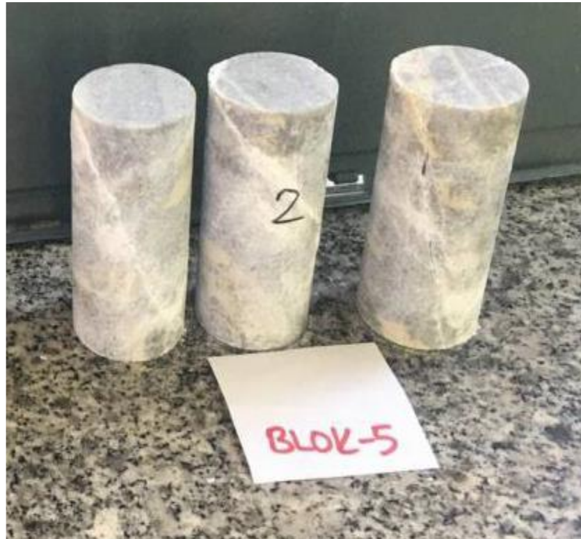
Figure 31. The view of the TCS test core samples after the testing
