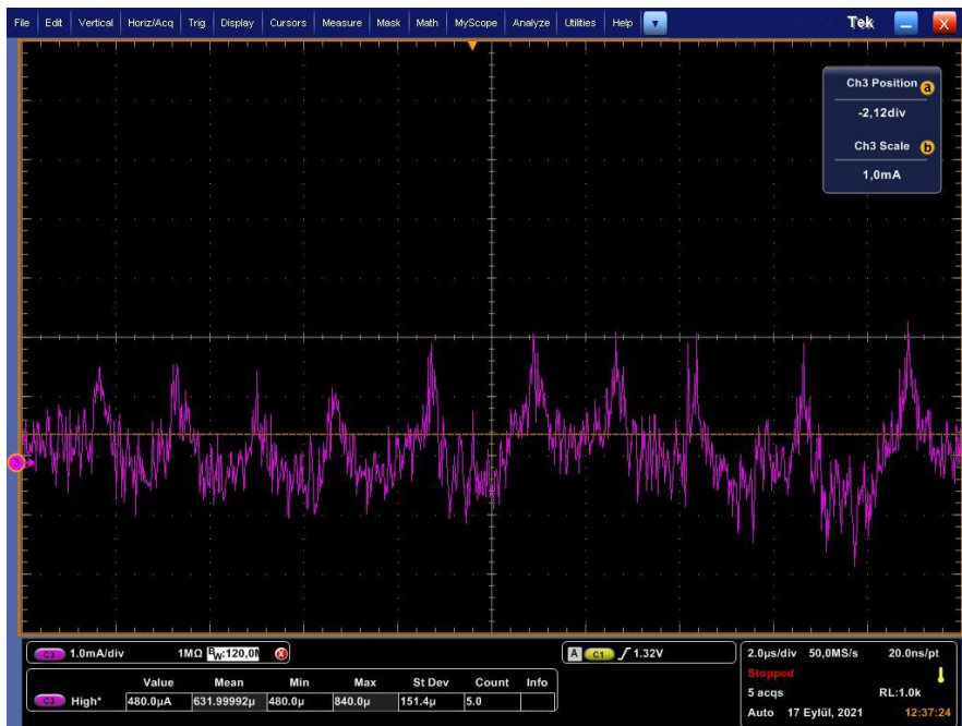
Figure 3.13 - Power Consumption of the Core for 2 us/div
