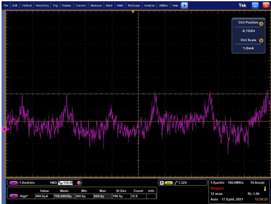
Figure 3.12 - Power Consumption of the Core for 1 us/div
