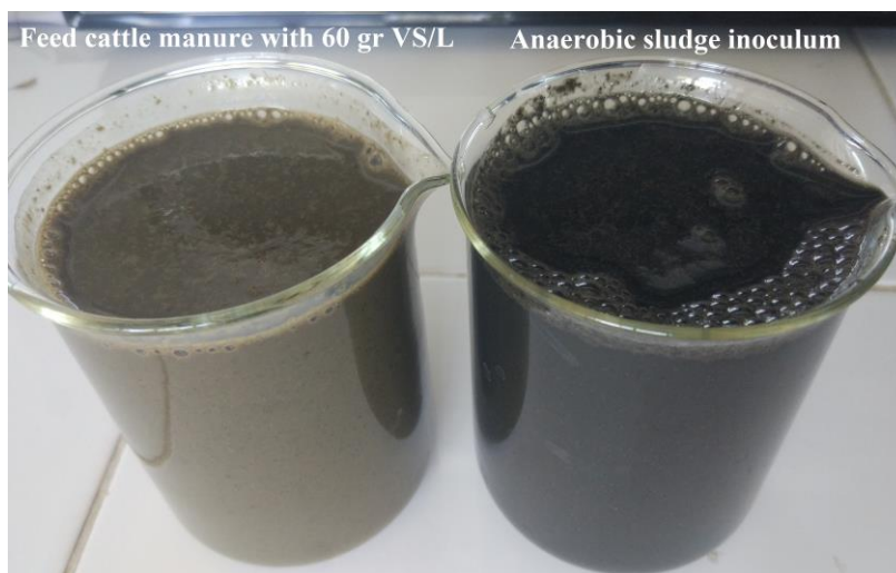
Figure 3.1. A photo of anaerobic sludge and feed cattle manure used in this study.
