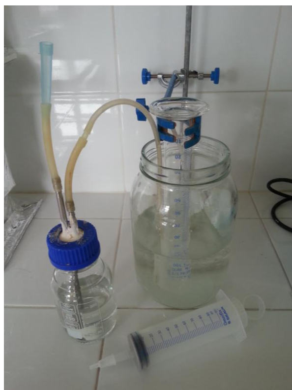
Figure 3.7. Water displacement method to measure the methane rate of the biogas.
