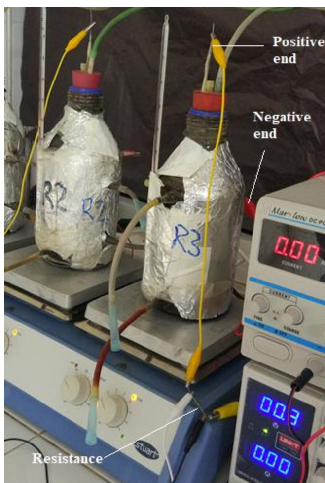
Figure 3.4. A presentation of the MEC+AD reactor's connection to the power supply unit. Three MEC+AD reactors and a control reactor were heated and stirred at 250-300 rpm by magnetic stirrers. The hoses and connection points of the hoses to the reactors were controlled for airtightness under water and soap foam by pumping air to the hoses and reactors. There were only two external power suppliers (Uni-T UTP 3315 TFL) that were
