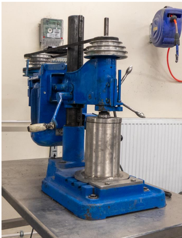
Figure 12. Laboratory Scale Vertical Stirred Mill and Stirrer Geometry
