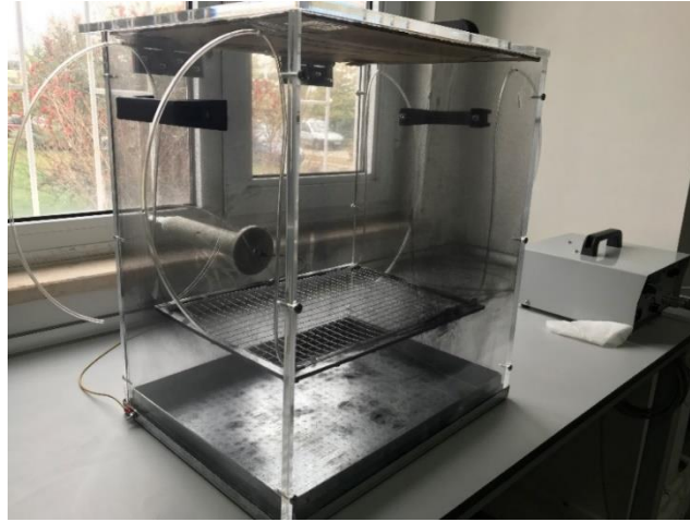
Figure 14 Commercial electrostatic flocking cabin.
