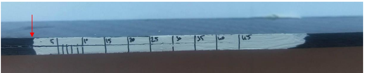
Figure 39 Painted DCB coupon.
