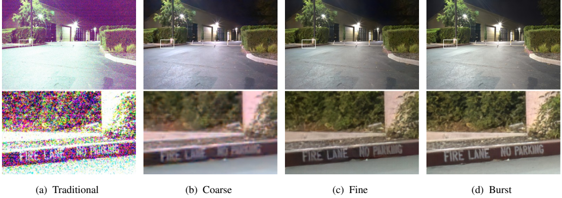
Figure 3.2. An example night photo captured with 0.1 sec exposure and its enhanced versions by the proposed coarse, fine and burst networks. As the cropped images demonstrate, the fine network enhances both the color and the details of the coarse result. The burst network produces even much sharper and perceptually more pleasing output.
