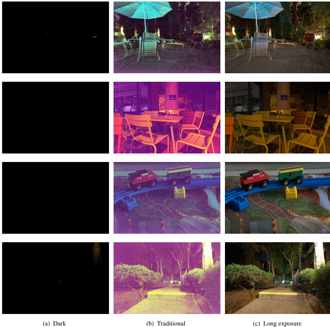
Figure 4.1. We show example (a) short exposure, dark raw images, (b) scaling and demosaicking dark images via traditional pipeline, (c) long exposure images from the SID dataset.
