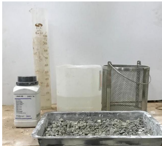
Figure 3.32. Test equipments prepared for aggregate soundness test
