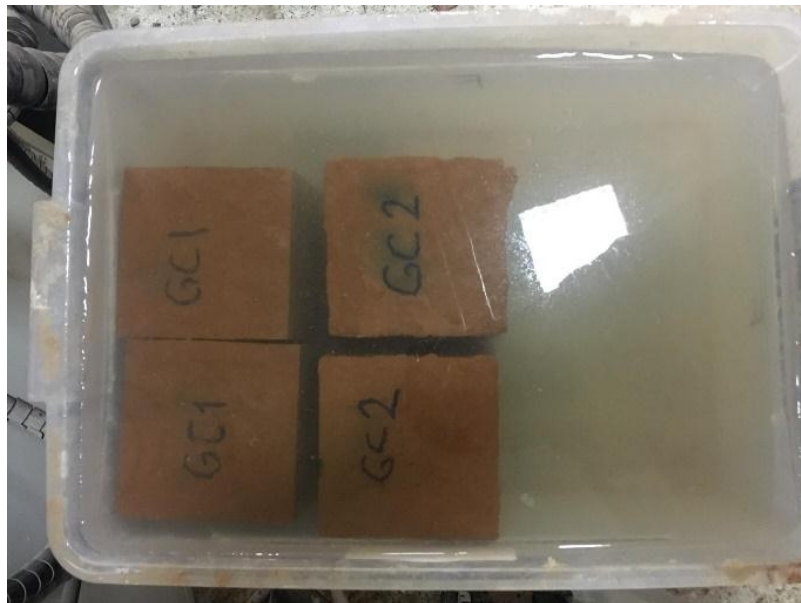
Figure 3.27. Geopolymer Concretes (in water curing GC1 and GC2 samples in final series)
