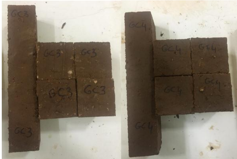
Figure 3.28. Geopolymer Concretes (GC3 and GC4 samples in final series)
