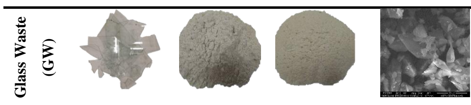
Figure 3.7. Glass waste images (from left to right; raw state, crushed state, ground state, SEM micrograph)
