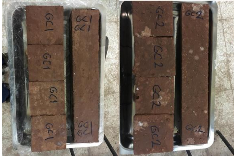
Figure 3.26. Geopolymer Concretes (GC1 and GC2 samples in final series)
