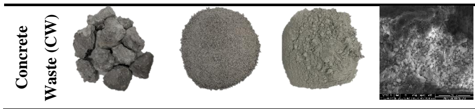
Figure 3.9. Concrete waste images (from left to right; raw state, crushed state, ground state, SEM micrograph)
