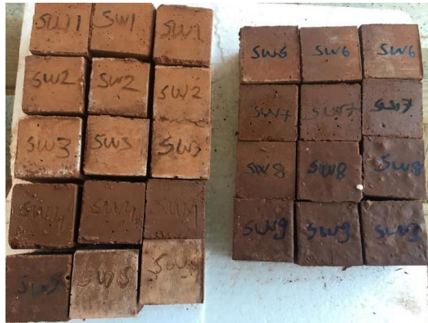
Figure 3.23. Geopolymer Mortars (Containing different proportions of CW, GW, HB, RCB, RT and Recycled Fine Aggregates)
