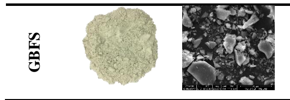
Figure 3.12. Granulated Blast Furnace Slag image (from left to right; raw state, SEM micrograph)
