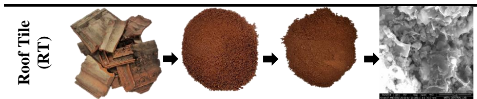
Figure 3.5. Roof tile images (from left to right; raw state, crushed state, ground state, SEM micrograph)
