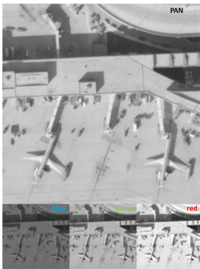
Figure 4.2. IQA PAN (top), blue (lower left), green (lower middle) and red (lower right) band image simulations for example EOIPL design, respectively.
