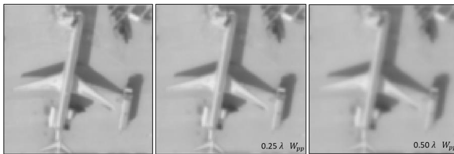
Figure 4.4. PAN band image simulations for EOIPL design (left), 0.25 peak to peak WFE (middle) and 0.5 peak to peak WFE (right) degraded image simulations, respectively.
