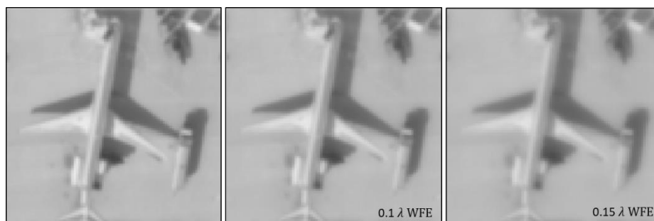
Figure 4.5. PAN band image simulations for EO IPL design (left), 0.10\lambda WFE (middle) and 0.15\lambda WFE (right) degraded image simulations, respectively.
