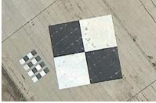
Figure 2.3.3.6. Knife edge targets are used for MTF and RER measurement from space [32].
