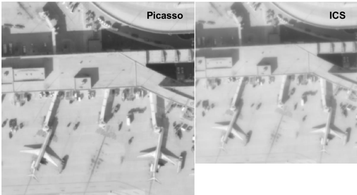
Figure 4.1. Image simulation outputs of IQA program for Picasso GENSAT1(left) and ICS GENSAT2 (right), respectively.
