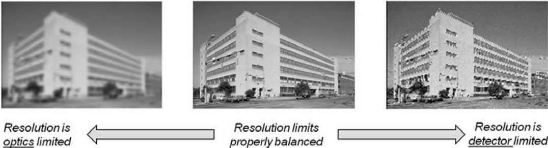
Figure 2.3.2.1. Balancing Q parameter in EOIPL design Characteristics of the image quality is depending on whether the spatial resolution is limited by optics or detector [14].
