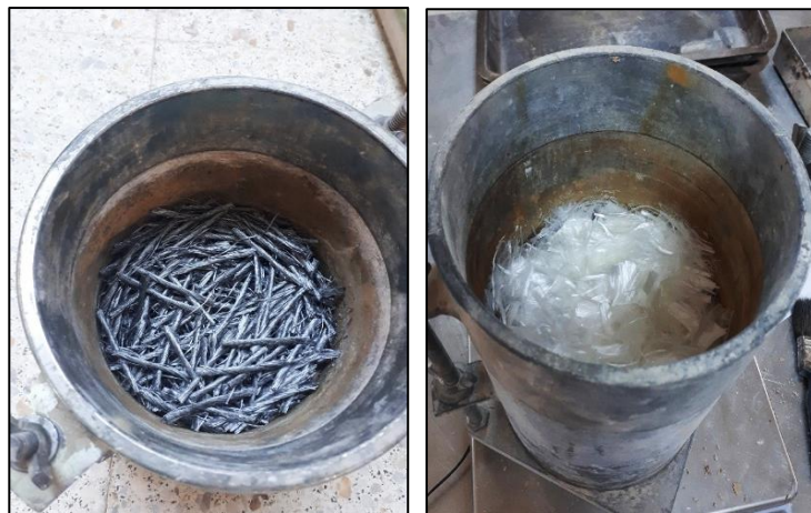
Figure 3.21 Synthetic fiber reinforcements that were placed between soil layers at h/4 depth.
