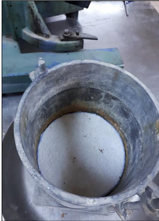
Figure 3.18 A geotextile reinforcement placed between soil layers.
