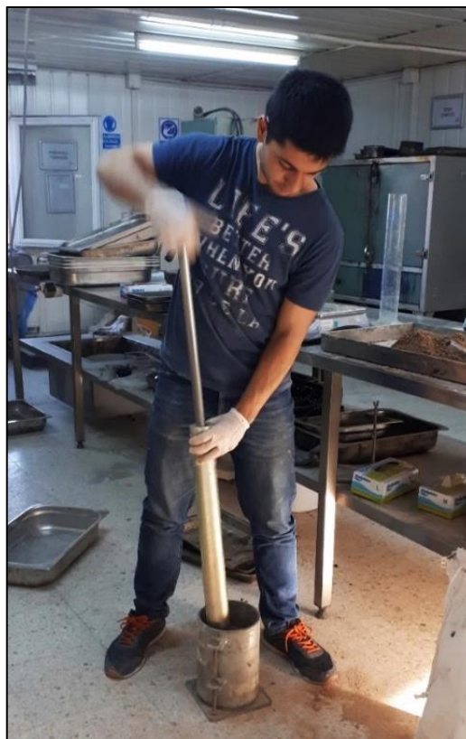
Figure 3.15 Compacting soil samples with 4.5 kg rammer.
