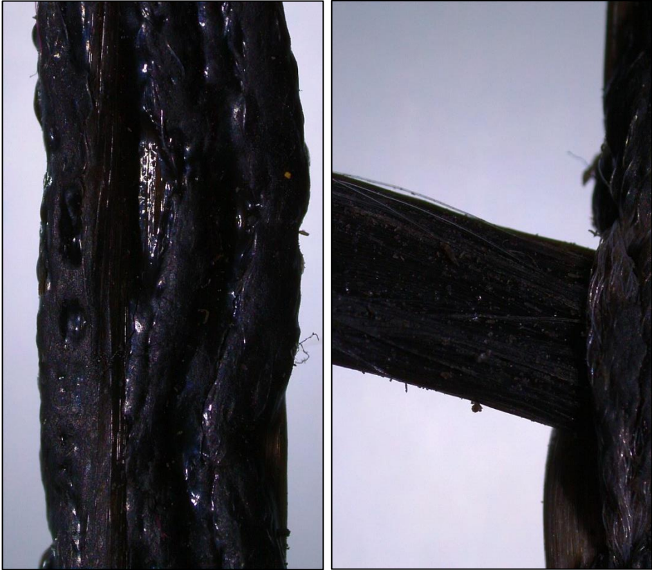
Figure 4.17 Images of Geogrid 1 under microscope.
