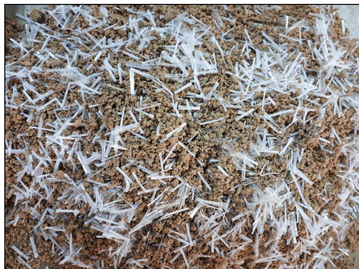
Figure 3.22 Fiber reinforcements and soil after mixed by hand.
