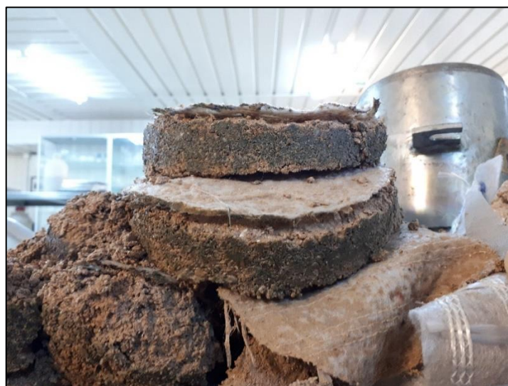
Figure 4.14 Soil layers and geotextiles that were extracted from the mold after CBR Test.
