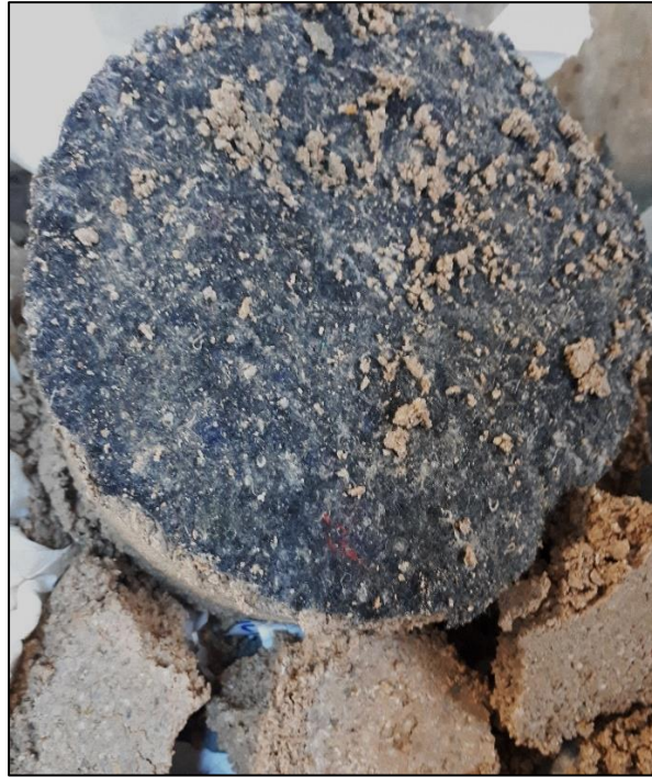
Figure 4.15 Condition of a geotextile reinforcement after CBR Test.
