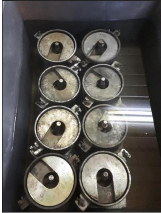
Figure 3.16 Compacted samples in the curing pool.
