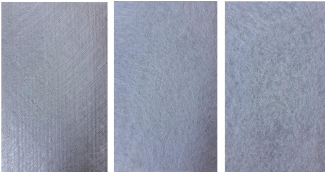
Figure 3.12 Surface textures of geotextiles; (a) Geotextile 12, (b) Geotextile 13, (c) Geotextile 14.
