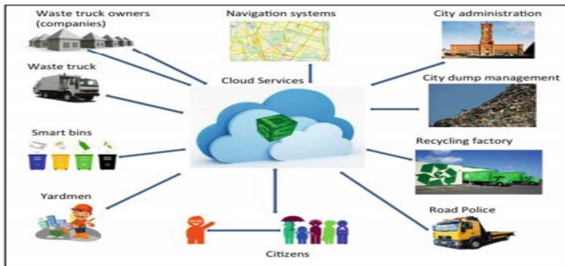
Figure 5.1. Smart Waste Management System Components [287].
