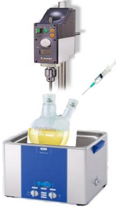
2,0 gr Kitosan + 20 mL isopropanol
