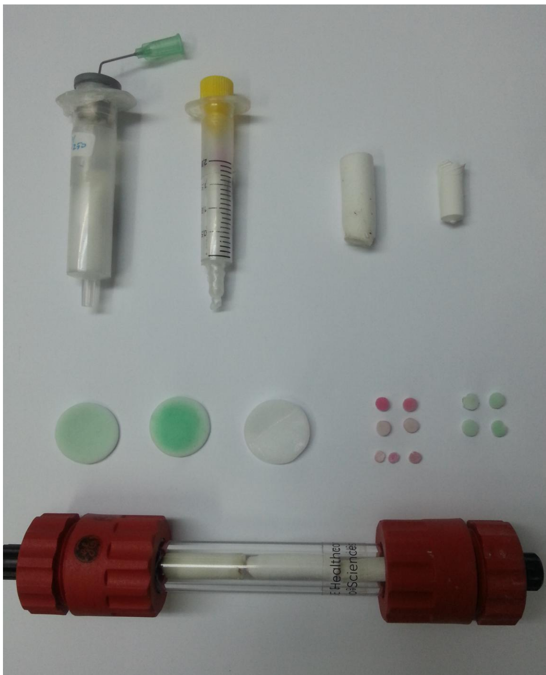
Figure 2.7. Production of cryogels in different forms.
