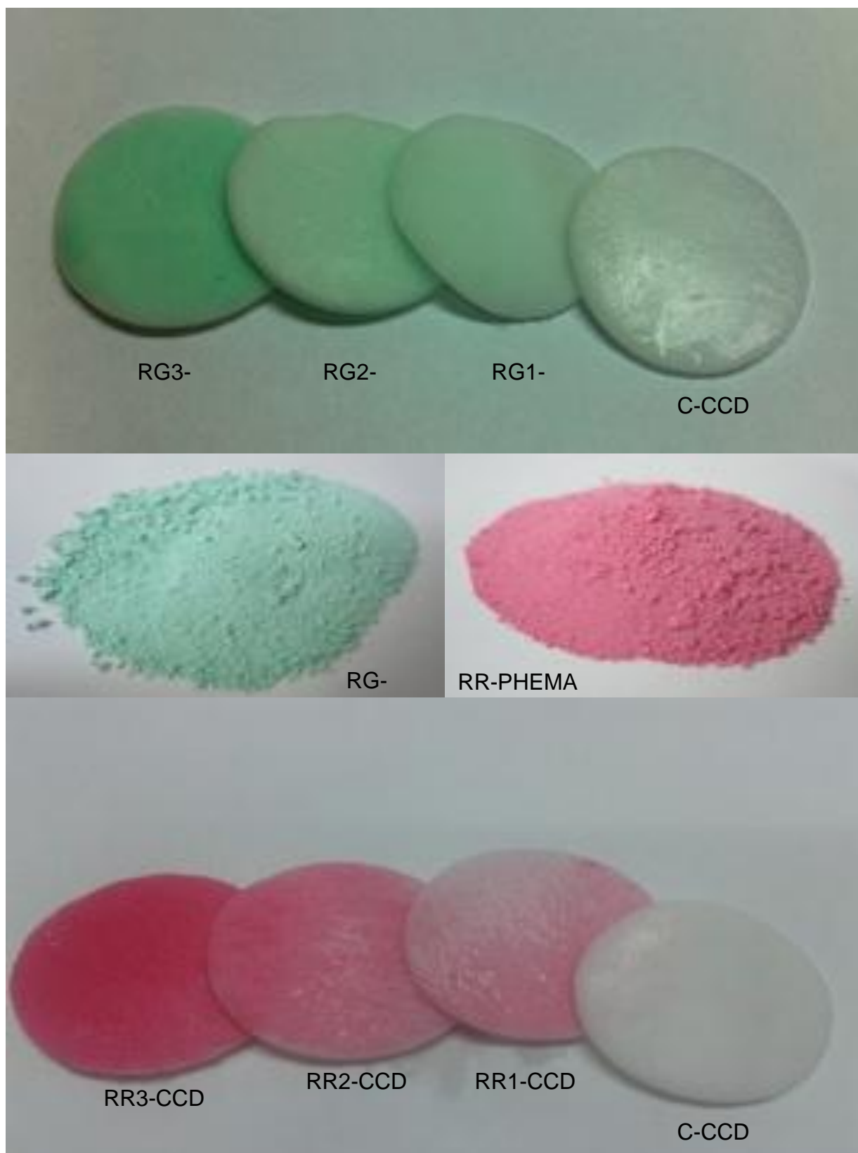
Figure 4.1. The optic photographs of the prepared CCD columns and RG and RR attached beads.
