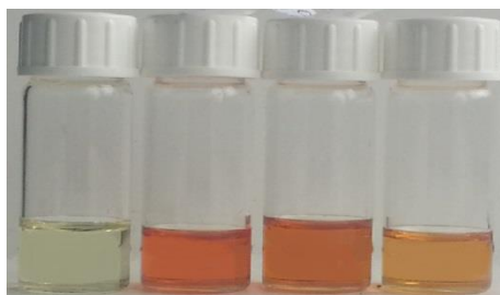
Figure 76: Colors of DMSO solutions of pure 37 and upon addition of 3:1, 1:1 and 1:3 mole ratios of \text{CN}^- from left to right
