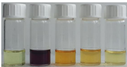
Figure 74: Colors of DMSO solutions of pure 37 and upon addition of 3:1, 1:1 and 1:3 mole ratios and an excess of OH^- from left to right
