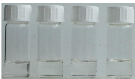
Figure 48: Colors of DMSO solutions of pure 34 and upon addition of 3:1, 1:1 and 1:3 mole ratios of \text{NO}_3^- from left to right
