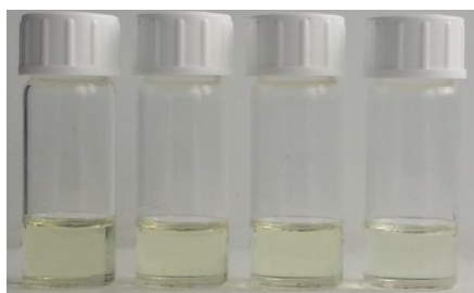
Figure 78: Colors of DMSO solutions of pure 37 and upon addition of 3:1, 1:1 and 1:3 mole ratios of \text{HSO}_4^- from left to right
