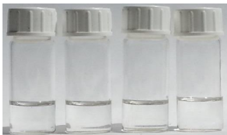
Figure 36: Colors of DMSO solutions of pure 33 and upon addition of 3:1, 1:1 and 1:3 mole ratios of \text{H}_2\text{PO}_4^- from left to right
