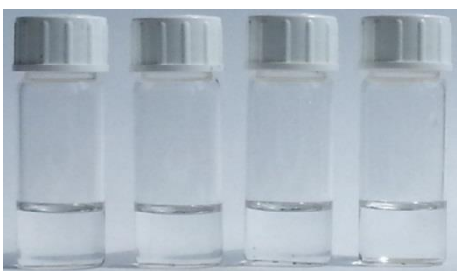
Figure 32: Colors of DMSO solutions of pure 33 and upon addition of 3:1, 1:1 and 1:3 mole ratios of \text{I}^- from left to right
