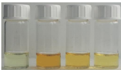
Figure 77: Colors of DMSO solutions of pure 37 and upon addition of 3:1, 1:1 and 1:3 mole ratios of \text{H}_2\text{PO}_4^- from left to right
