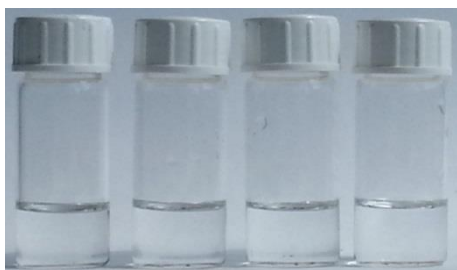
Figure 31: Colors of DMSO solutions of pure 33 and upon addition of 3:1, 1:1 and 1:3 mole ratios of \text{Br}^- from left to right
