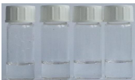
Figure 91: Colors of DMSO solutions of pure 40 and upon addition of 3:1, 1:1 and 1:3 mole ratios of Cl^- from left to right
