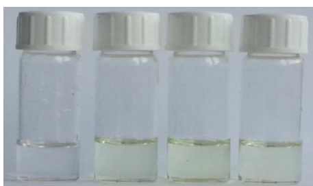
Figure 94: Colors of DMSO solutions of pure 40 and upon addition of 3:1, 1:1 and 1:3 mole ratios of \text{OH}^- from left to right
