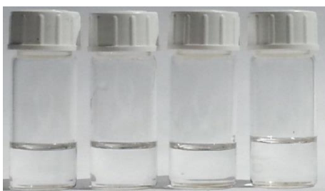
Figure 37: Colors of DMSO solutions of pure 33 and upon addition of 3:1, 1:1 and 1:3 mole ratios of \text{HSO}_4^- from left to right
