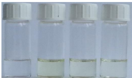
Figure 55: Colors of DMSO solutions of pure 35 and upon addition of 3:1, 1:1 and 1:3 mole ratios of \text{CN}^- from left to right
