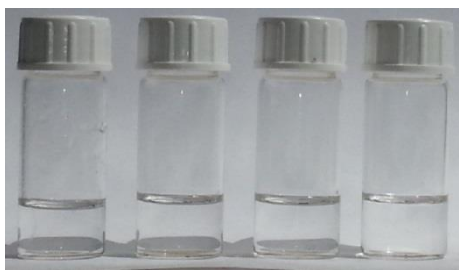
Figure 92: Colors of DMSO solutions of pure 40 and upon addition of 3:1, 1:1 and 1:3 mole ratios of \text{Br}^- from left to right
