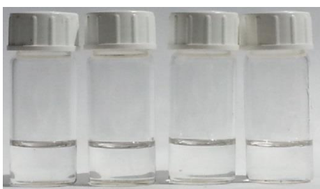
Figure 35: Colors of DMSO solutions of pure 33 and upon addition of 3:1, 1:1 and 1:3 mole ratios of \text{CN}^- from left to right
