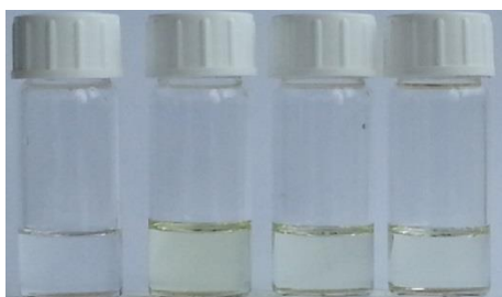
Figure 56: Colors of DMSO solutions of pure 35 and upon addition of 3:1, 1:1 and 1:3 mole ratios of \text{H}_2\text{PO}_4^- from left to right
