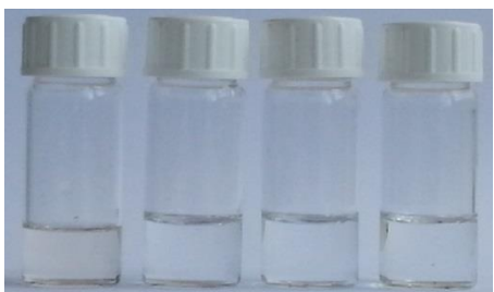
Figure 83: Colors of DMSO solutions of pure 39 and upon addition of 3:1, 1:1 and 1:3 mole ratios of \text{I}^- from left to right
