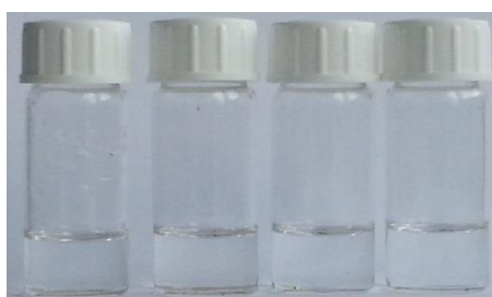
Figure 93: Colors of DMSO solutions of pure 40 and upon addition of 3:1, 1:1 and 1:3 mole ratios of \text{I}^- from left to right
