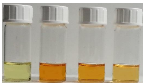
Figure 75: Colors of DMSO solutions of pure 37 and upon addition of 3:1, 1:1 and 1:3 mole ratios of OAc^- from left to right
