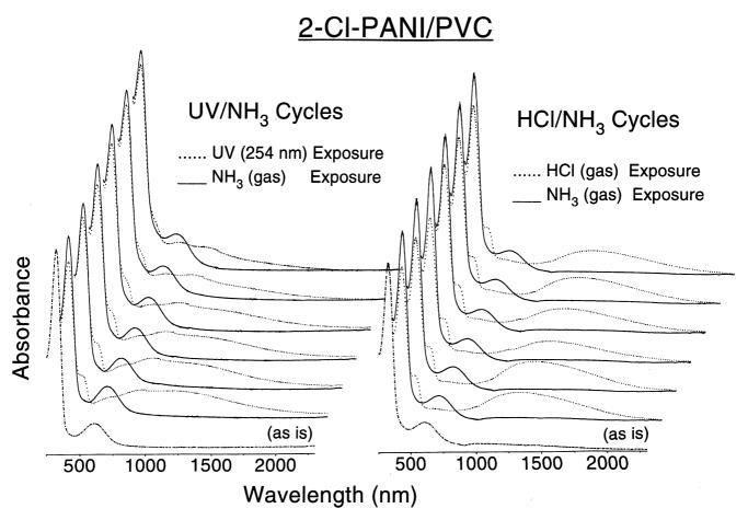
Fig. 4. UV–Vis–NIR spectra of the 2-Cl-PANI/PVC composite films exposed to UV/NH<sub>3</sub> and HCl/NH<sub>3</sub> cycles.
