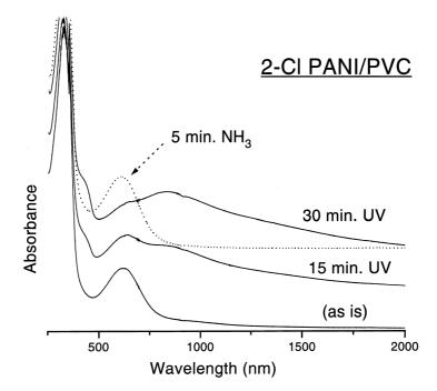
Fig. 1. UV–Vis–NIR spectra of 2-Cl-PANI/PVC composite films before and after 15 and 30 min exposure to UV and after further exposing them to 5 min of NH<sub>3</sub> vapours.
