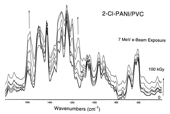
Fig. 3. FTIR spectra of 2-Cl-PANI/PVC composite films before and after exposure to 7 MeV e-beams.
