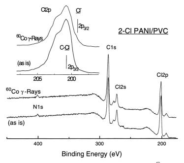
Fig. 2. XPS spectra of 2-Cl-PANI/PVC composite films before and after 200 kGy  $^{60}$ Co  $\gamma$ -rays exposure.
