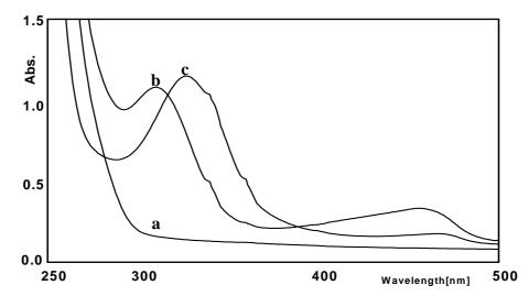
**Figure 1.** UV-vis spectra of (a) thiophene-HBF<sub>4</sub> mixture (1:1), (b) pyrrole-HBF<sub>4</sub> mixture (1:1), (c) thiophene-pyrrole-HBF<sub>4</sub> mixture (1:1:2), (The concentrations of species, C = 0.001M).
