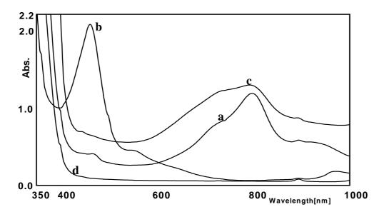
**Figure 2.** UV-vis spectra of (a) pyrrole-FeCl<sub>3</sub> mixture (1:1), (b) pyrrole-thiophene-HBF<sub>4</sub>-FeCl<sub>3</sub> (1:1:2:2) mixture, (c) pyrrole-thiophene-FeCl<sub>3</sub> (1:1:2), (d) thiophene-FeCl<sub>3</sub> mixture (1:1) (The concentrations of species, C=0.001M).
