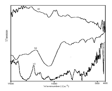
**Figure 5.** Infrared spectra for (a) polypyrrole, (b) sample B prepared from B solution that contains 0.01 mol pyrrole, 0.01 mol thiophene and 0.02 mol HBF<sub>4</sub>, (c) polythiophene prepared electrochemically.
