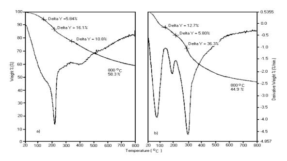
**Figure 3.** TGA curves for (a) polypyrrole homopolymer, (b) sample B prepared from B solution that contains 0.01 mol pyrrole, 0.01 mol thiophene and 0.02 mol HBF<sub>4</sub>.
