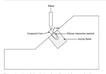
**Figure 1** Use of the device that allowed fracture loading at 135° to the long axis of the specimen.
