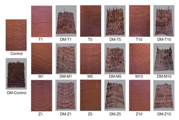
**Fig. 5.** Stereomicroscope images and depth map presentations of tooth surfaces treated with diamond burs used after three different specimens and 1, 5, and 10 times preparations. In depth maps, peaks represent rougher areas.
