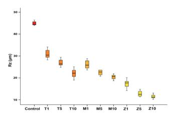
Fig. 3. Mean roughness value of each group with increase in number of cuts.
