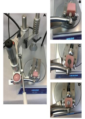
**Fig. 1.** (A) Modified milling machine for preparations, (B) Magnified view of the diamond bur position on tooth specimen, (C) Magnified view of the diamond bur position on CoCr specimen, (D) Magnified view of the diamond bur position on zirconia specimen.
