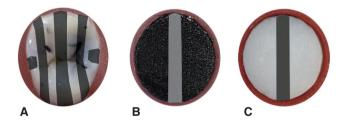
**Fig. 2.** (A) Preparation (five cuts) on tooth sample, (B) Preparation (one cut) on CoCr (DMLS) sample, (C) Preparation (one cut) on zirconia sample.
