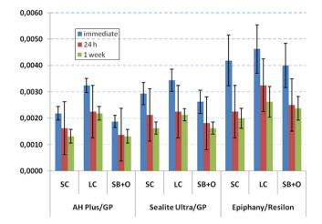
Figure 2 Fluid conductance values  $(L/minute/cmH_2O)$  of test specimens with respect to the post space preparation time (immediately, at 24 hours, and at 1 week) and filling technique. GP = gutta-percha; LC = lateral compaction; SB = system B/Obtura; SC = single cone.
