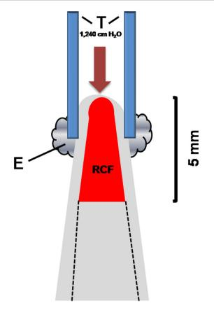
**Figure 1** Schematic view of a specimen attached to the fluid filtration setup. An arrow indicates the direction of water movement. E = epoxy resin; RCF = root-canal filling; T = tube.
