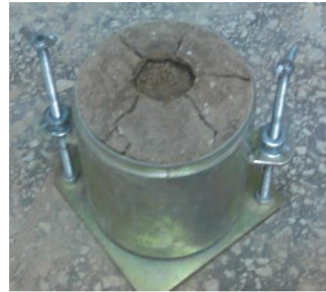
FIGURE 10: The view of 25% FA mixes sample after the CBR test.
