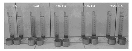
Fig. 4. Tubes of free swell index tests.
