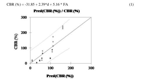
Fig. 7. Measured and predicted CBR values derived from Eq.1.
