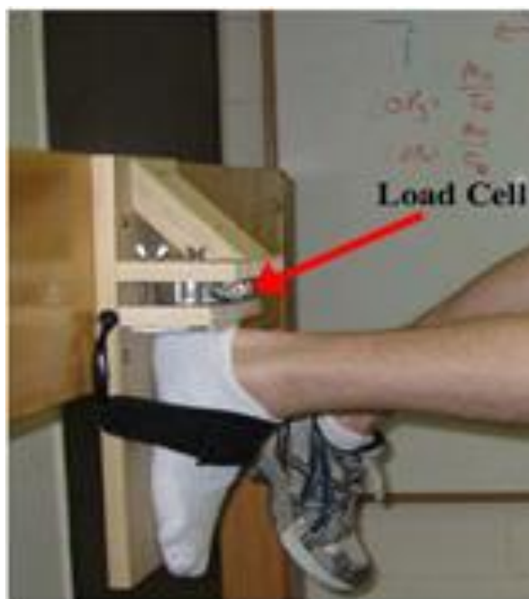
Figure 2.10. Example for the measurement of hamstring force with load cell placed on the back side of calcaneus.
