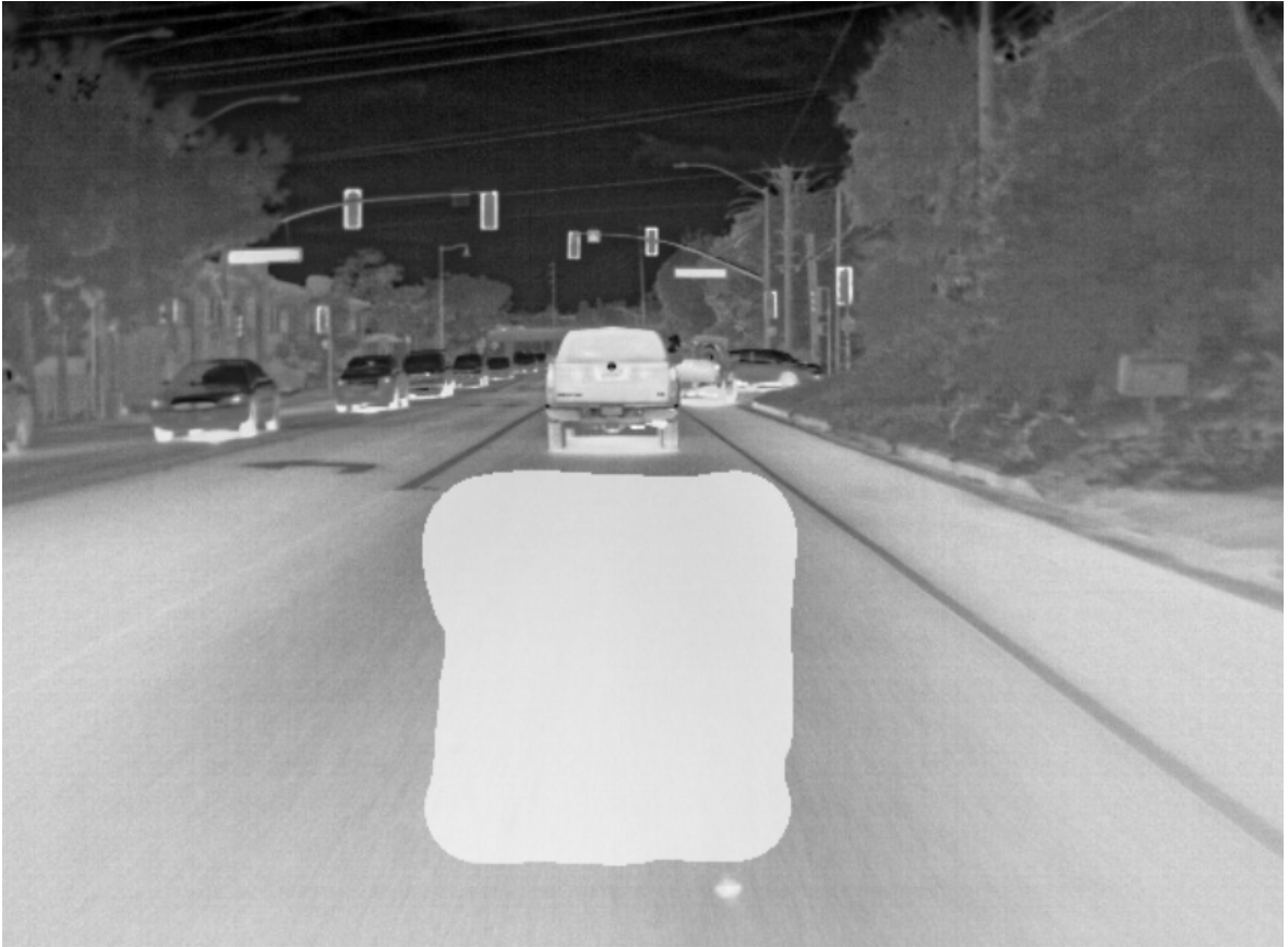
Figure 4.2 The process of masking where the object will be generated during inpainting with stable diffusion.
