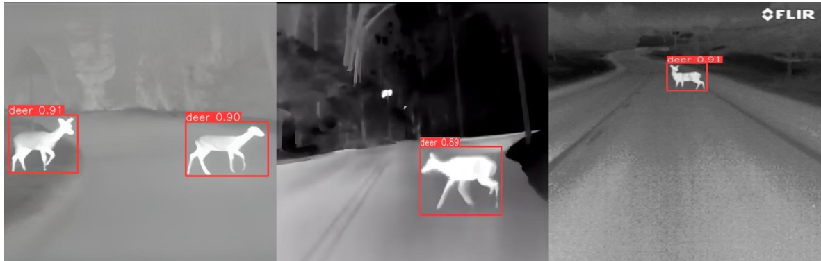
Figure 5.7 This image represents the detection results of the model trained with the generated dataset on real-world corner case images.
