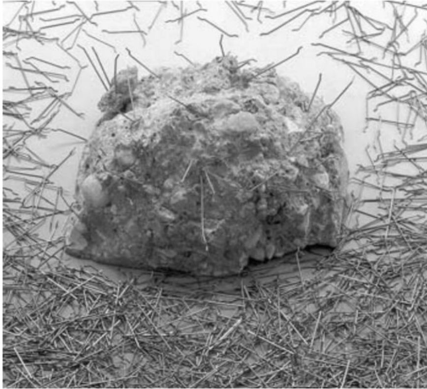
Figure 2.4 Steel fibers and steel fiber reinforced concrete. Adapted from (Kolymbas, 2019)
